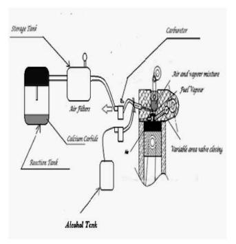
Fig. 1:- Schematic diagram of the total experimental setup.
